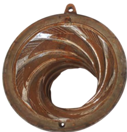
Lining for Simo® grinder before refurbishment
